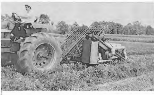
Figure 3. Front view of 1971 combination peanut digger-salvager. View of cleaning fan, inclined conveyor and bagging attachment as installed on the left side of the machine.
