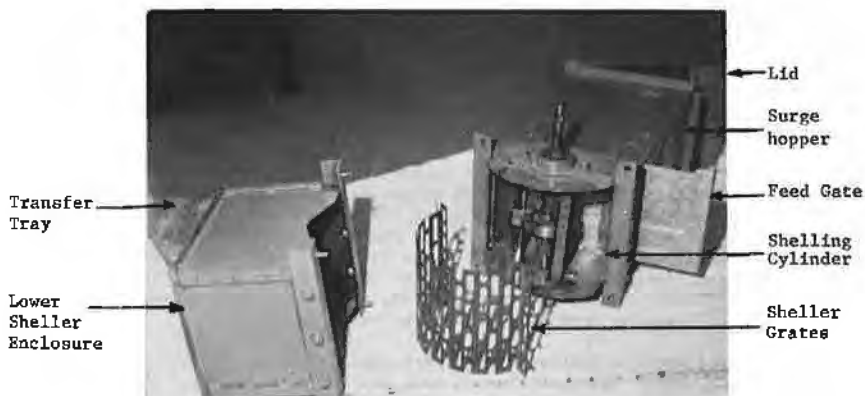
Figure 2.--The general design of the model 2 sheller
