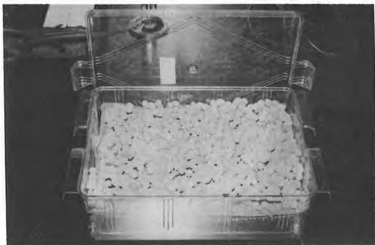
Figure 1. Method for experimental storage of peanuts in controlled relative humidity and temperature.
