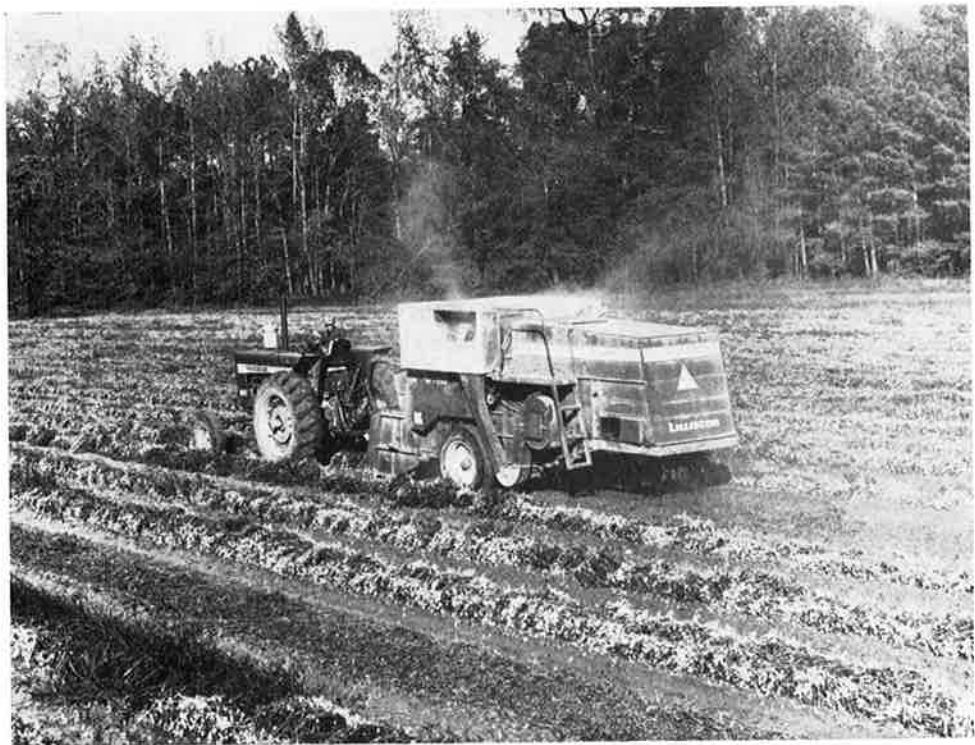
Figure 15. Tractor Powered Peanut Combine with Bulk Holding Tanks for the Picked Nuts.
