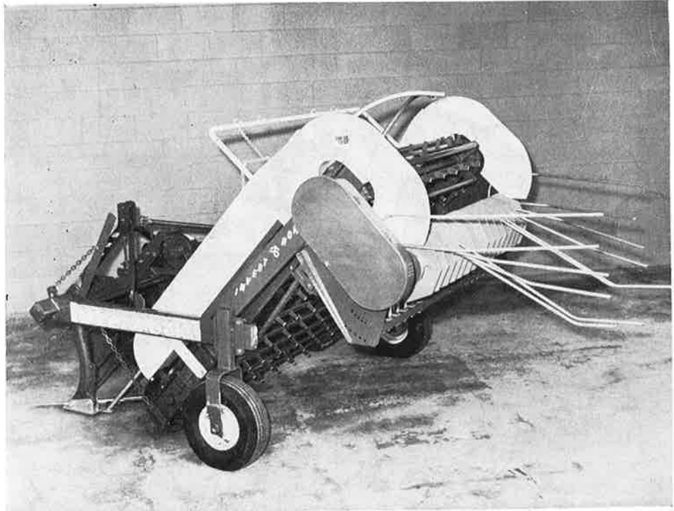
Figure 14. Tractor Powered Digger-Shaker-Windrower that Inverts the Plant.
