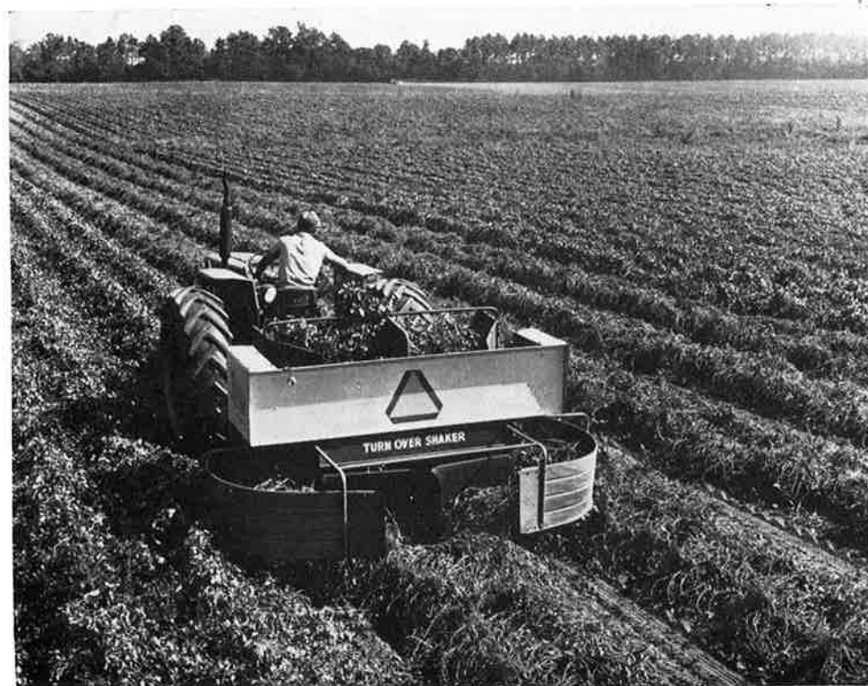
Figure 9. Inverted Plants Place Pods in Improved Curing Environment.
