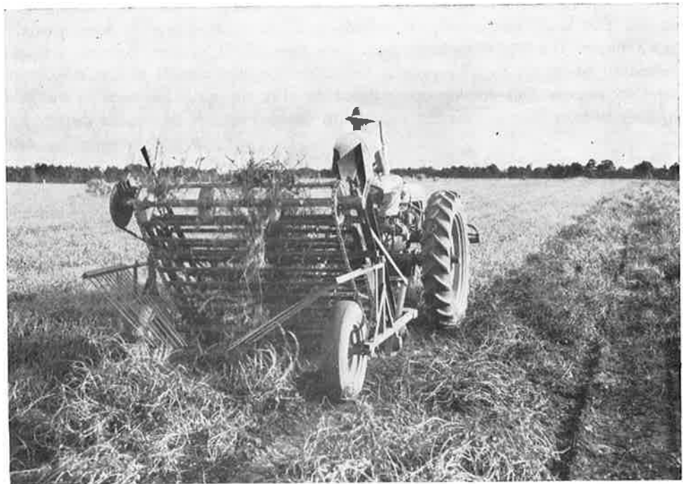
Figure 6. Equipment Was Developed in the Late 1940's to Shake Out the Dirt and Windrow the Plants.
